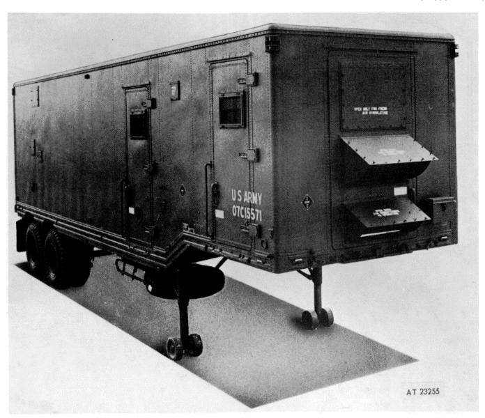
Figure 1-16. Semitrailer, van petroleum testing laboratory, XM822-rightfront view
