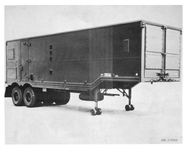
Figure 1-7. Semitrailer, van: electronic, XM680-right front view.
