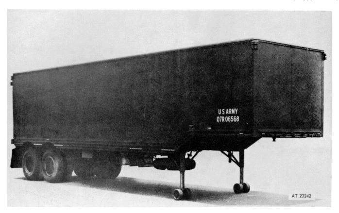
Figure 1-18. Semitrailer, van teletype, XM823-rightfront view
