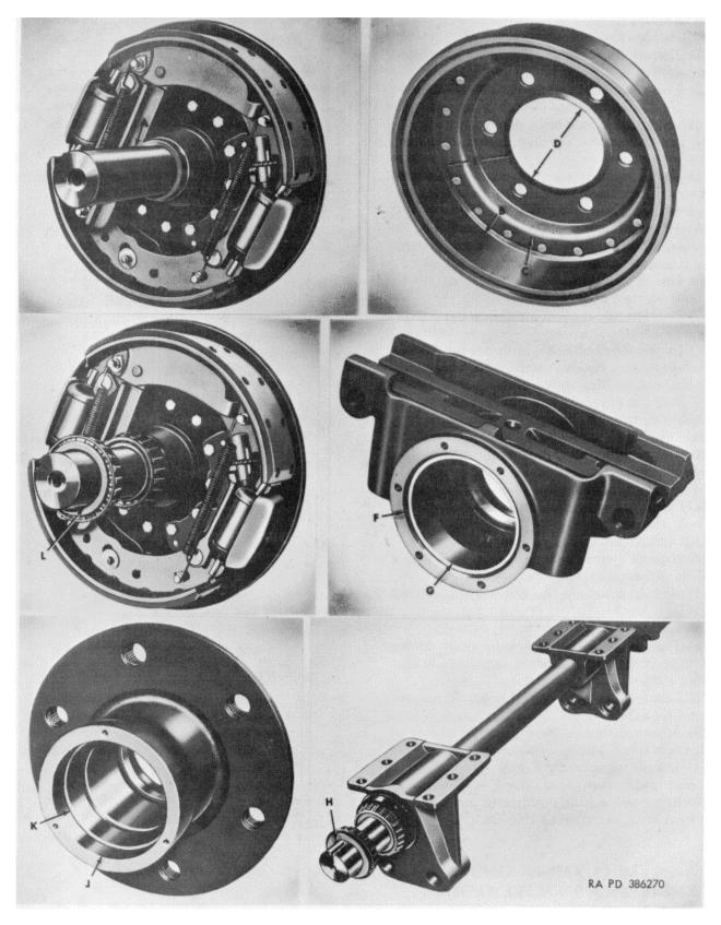
Figure 6-1. Standard repair measurement points
