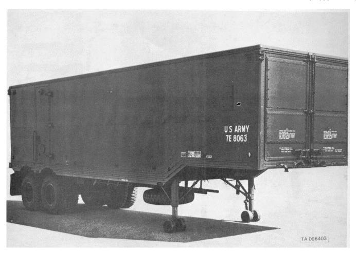
Figure 1-9. Semitrailer, van electronic, XM680E1-right front view.
